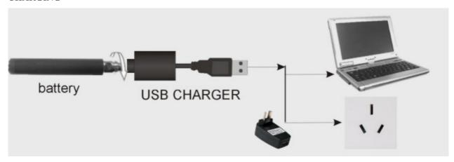
To charge a battery, screw the battery into the USB charger. After that, plug the USB charger into the wall charger (AC charger) or connect the USB charger to your computer. The charging time is 1-3 hours (depending on how the battery is charged already). At the beginning of charging, the battery will signal by blinking a few times. During charging, the light on the USB module is red. Once the battery is charged, the light will change from red to green.
